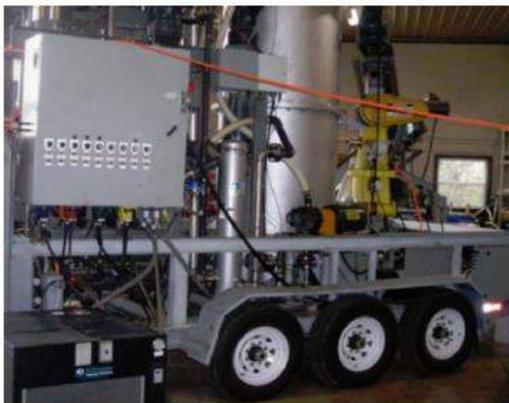
Mobile pyrolysis unit that converts poultry litter to biochar and heating oil;
